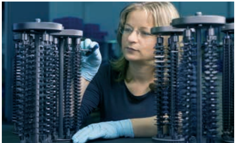
The tools are coated in an optimal fashion in the production line for indexable inserts by using various combinations of pre- and post-treatment methods, coating materials, and tolerances.
