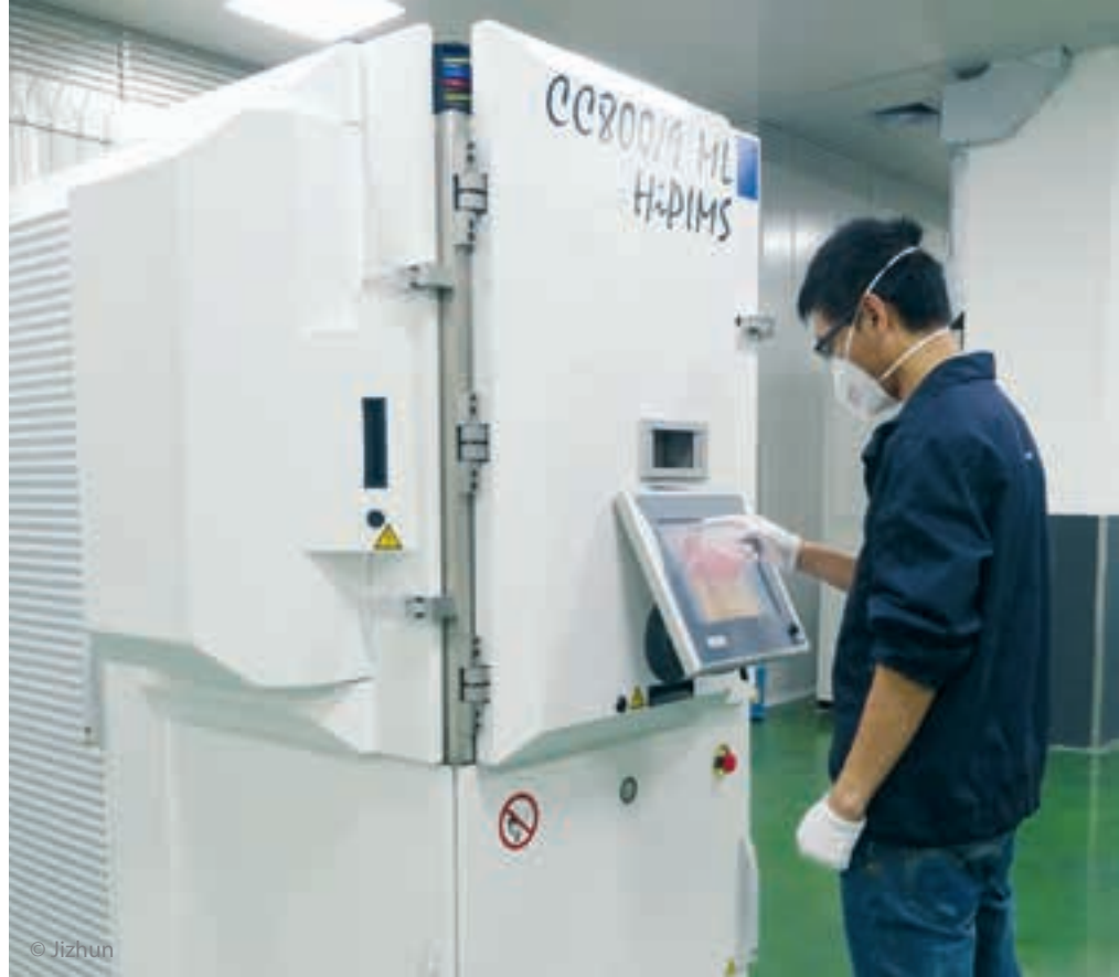
The CC800®/9 ML HiPIMS is a combination of HiPIMS and DC technology.
