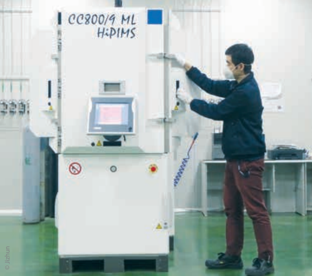
The CC800®/9 ML HiPIMS deposits hard, tough, oxidation-resistant and highly adhesive coatings.
