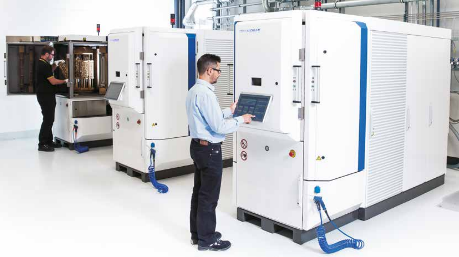
Three CC800® HiPIMS systems are now in use on a daily basis at Horn's own coating center. (Photo: Horn)
