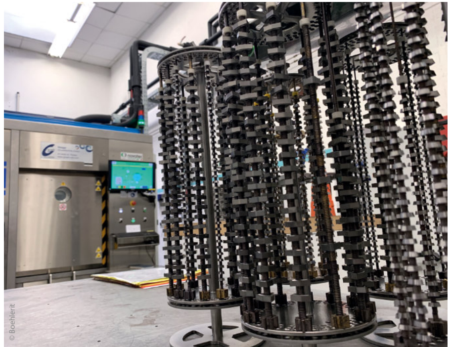
Broad innovation and investment offensive at Boehlerit: the new cleaning system optimally prepares the inserts for coating.
